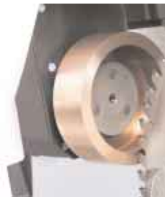
working position of the rotary electrode at the circumference of the saw blade
