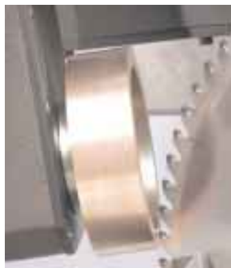
working position of the rotary electrode on the chamfer facet of the PCD saw blade
